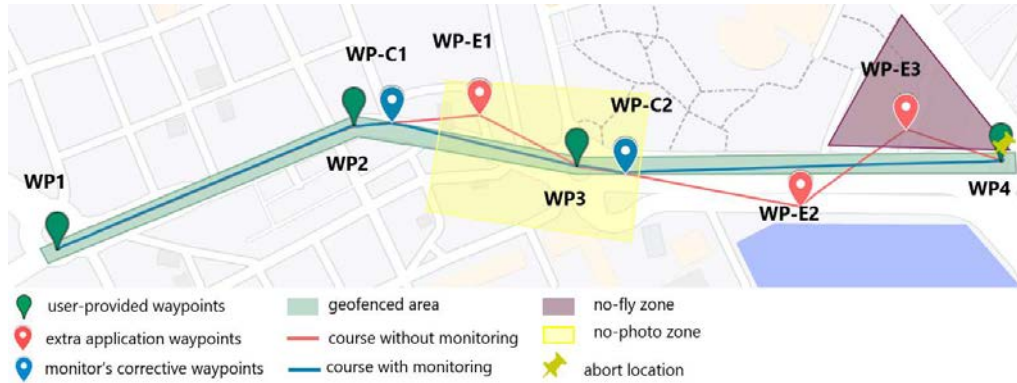
FIGURE 7.8: Simulation experiment with the monitoring mechanism disabled (red line) vs enabled (blue line)
