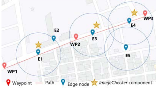
(A) Waypoints of the application Navigator and deployment of the ImageChecker on the edge nodes
